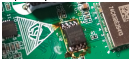
Fig. 15. Sample traces after manipulations with the memory chip
