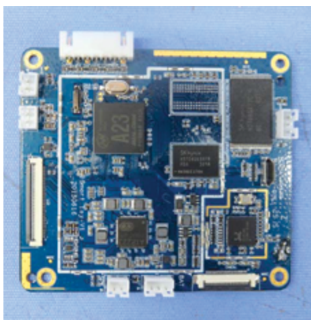
Fig. 18 The motherboard of the Smart Toy with the USB port
