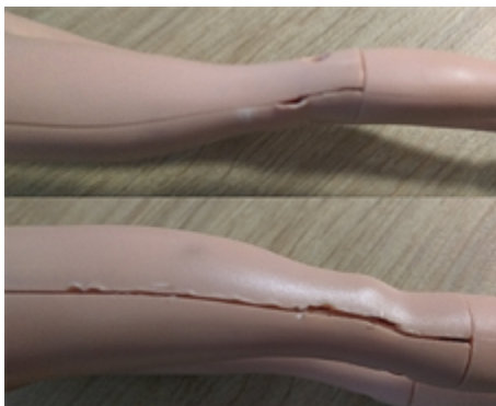
Fig. 12 Traces left when a Hello Barbie doll has been opened
